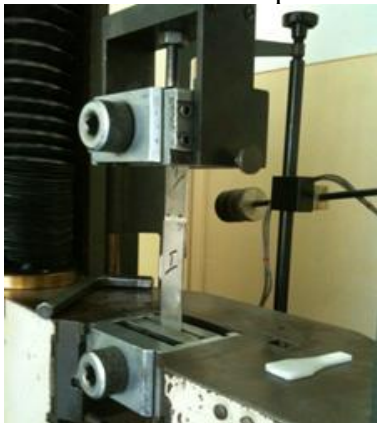
Figure 8. Clamping the sample assembly in the type traction device HECKERT FPZ 100
