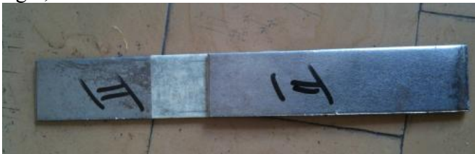
Figure 6. Assembly made in order to carry out the shear test [14] (normal view).
