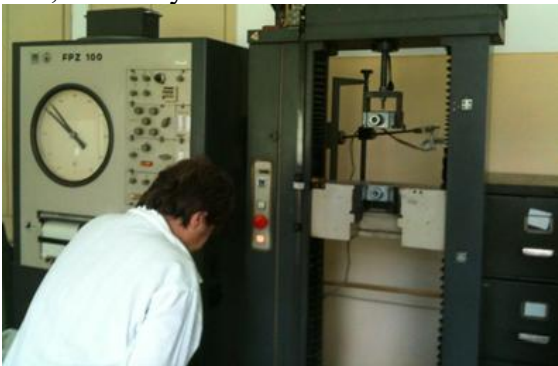
Figure 7. Shear tests HECKERT FPZ 100 machine
